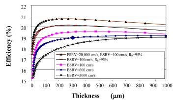
Figure 5: Simulated curves of screen-printed solar cell efficiency plotted as a function of (a) base thickness and BSRV.
