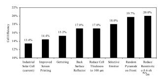
**Figure 1** Technology roadmap to achieve 20%-efficient solar cells using a combination of manufacturable technologies.
