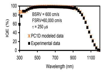
Figure 4: Measured and simulated IQE over the entire wavelength for the 19.0% FZ Si cell.
