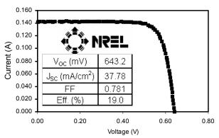
Figure 2 I-V measurements by NREL for the 19% textured front and back 100  $\Omega$ /sq emitter cell on 0.6  $\Omega$ -cm FZ Si.
