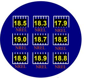
Figure 3 The distribution of nine 4 cm<sup>2</sup> cells with a 3.8 cm<sup>2</sup> mask on a 4 inch 0.6  $\Omega$ -cm FZ wafer textured on both sides.
